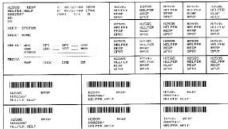
This example shows one label format that prints 22 labels at once; each line indicates a cut between labels. For this health care application, duplicate labels are essential to tracking samples.
